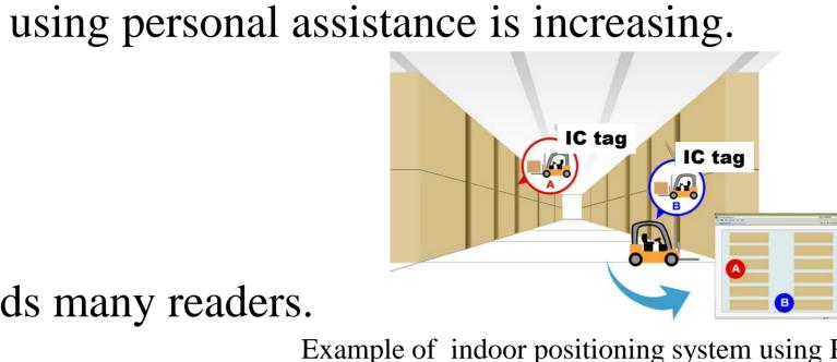
Example of indoor positioning system using RFID (AirLocation:Hitach corp.)
